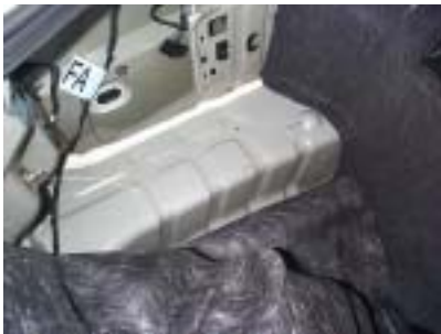
Partially remove carpet from work area.
